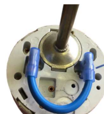
Figure 4.2 Bridging wire fitted to TSE Thermostat
