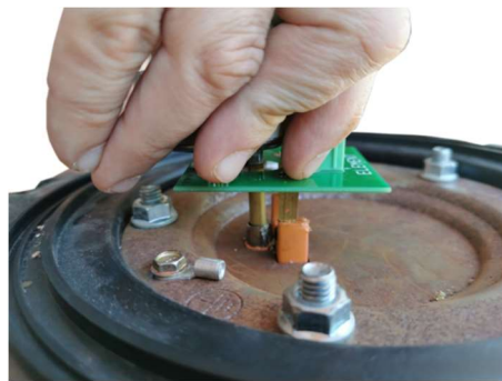
Figure 4.8 Thermostat & element adapter plugged into element
