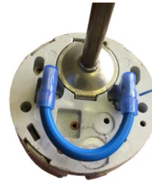
Figure 4.4 Bridging wire fitted to TSE Thermostat
