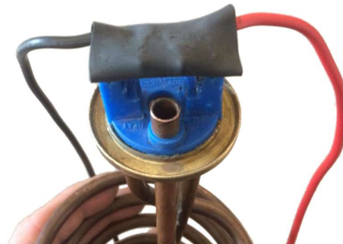
Figure 4.6 Element connector fitted to flange-type element
