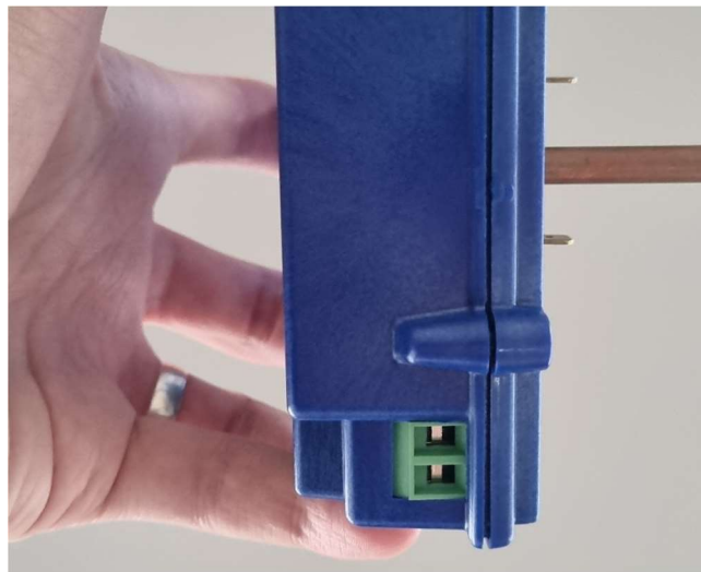
Figure 4.5. STEP 12b: Rotate the Elon Smart 90° in the thermostat pocket to make the AC wires easier to insert.
