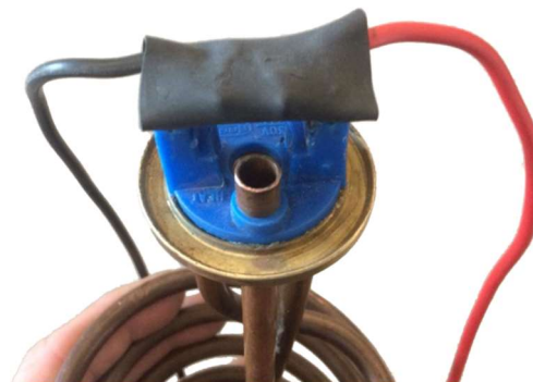
Figure 4.6 Element connector fitted to flange-type element
