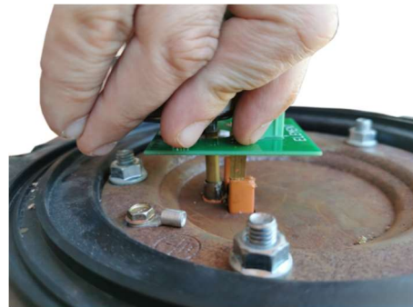
Figure 4.8 Thermostat & element adapter plugged into element
