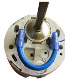
Figure 4.4 Bridging wire fitted to TSE Thermostat
