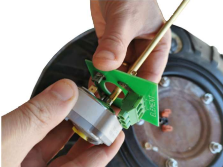
Figure 4.7 Thermostat plugged into element adapter
