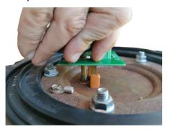
Figure 4.8 Thermostat & element adapter plugged into element
