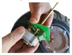
Figure 4.7 Thermostat plugged into element adapter
