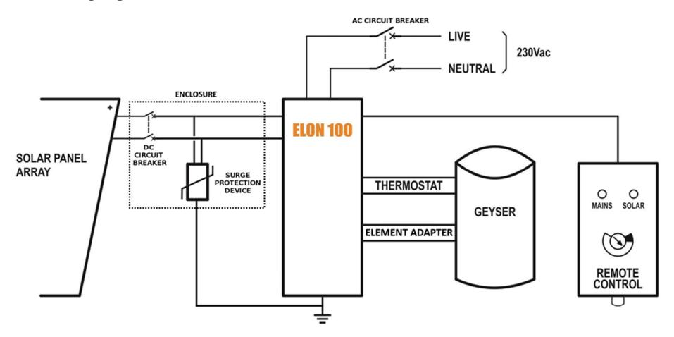
Note 1: Both AC & DC circuit breakers or isolators must be installed within 1.5m of the geyser (water heater), line of sight.
