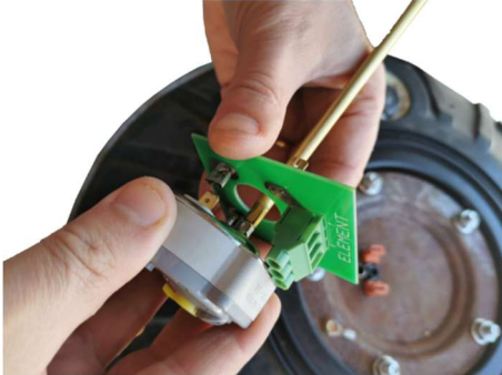
Figure 4.7 Thermostat plugged into element adapter
