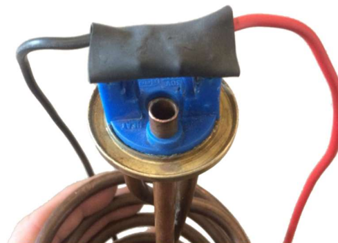
Figure 4.6 Element connector fitted to flange-type element
