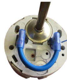
Figure 4.4 Bridging wire fitted to TSE Thermostat
